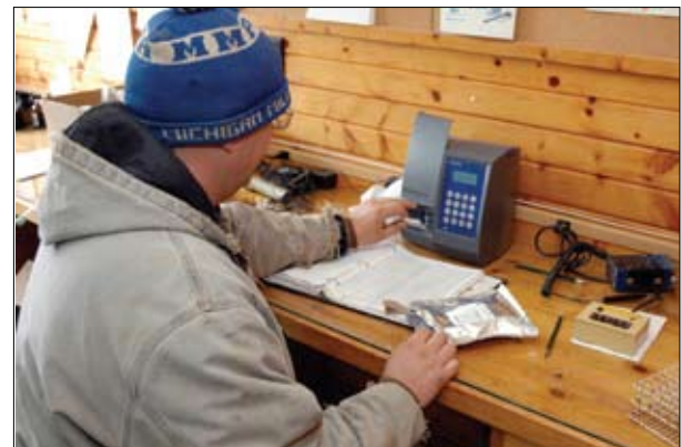
The dairy farm staff says the DeLaval SCC tester is a great tool for quickly identifying high count cows and for learning when cows are back to normal.
