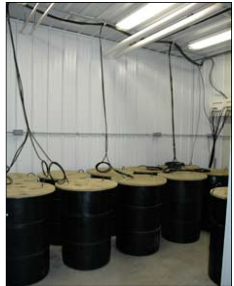
Excretions from the animals are stored in these containers to simulate manure storage. Emissions from the barrels are also monitored.
